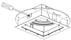
3 Tighten screw to lock adapter plate in place.
