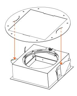
1 Make sure the spring clips on the housing line up with indicators shown on the adaptor plate.
